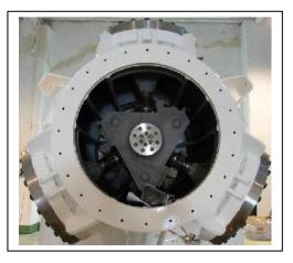
In addition, in case of black out or another fault, the same electromechanical control system, thanks to an internal security device, allows the emergency closing of the blades in "flag" mode, so the rotations can be stopped in just 0.8 seconds.
